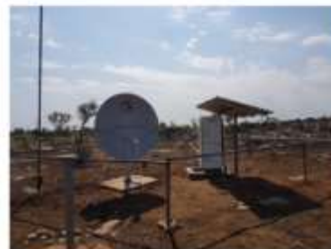
Image courtesy of Geoscience Australia. Image outlines an on-site setup of a seismic monitoring station.
