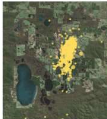
Distribution of aftershocks recorded following the 16 September 2018 Lake Muir earthquake. Source: Geoscience Australia
