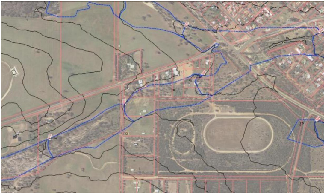
Extract from Figure 13E Katanning Flood Assessment Opus 2014 showing 'Extent of Flood Area –Flood Level Contours at 2m intervals'
