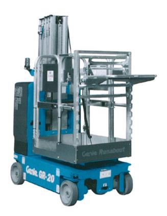
This unit is self-propelled single person platform that will rise to a working height of 6.47 meters. At 975 kg (spread over four rubber wheels) it is unlikely to damage the gallery floor. A safety harness is included free of charge for work beyond 2 meters.
